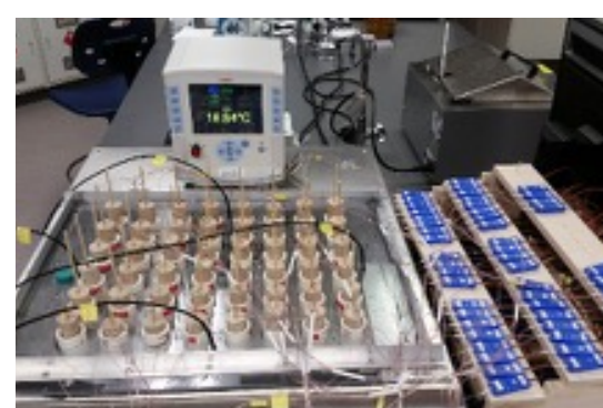
Figure 4. Heat treatment water bath for determining the specific lethal dose for forest product pests at the Pacific Forestry Centre (photo by Meghan Noseworthy, NRCan)
