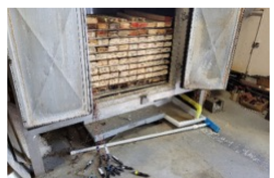
Figure 5. Experimental testing using a lab kiln for heat treatment of sawn green wood at 52 °C for 30 minutes to determine minimum lethal temperatures for pinewood nematode Bursaphelenchus xylophilus (photo of experimental kiln at FPIInnovations by Angela Dale, NRCan)
