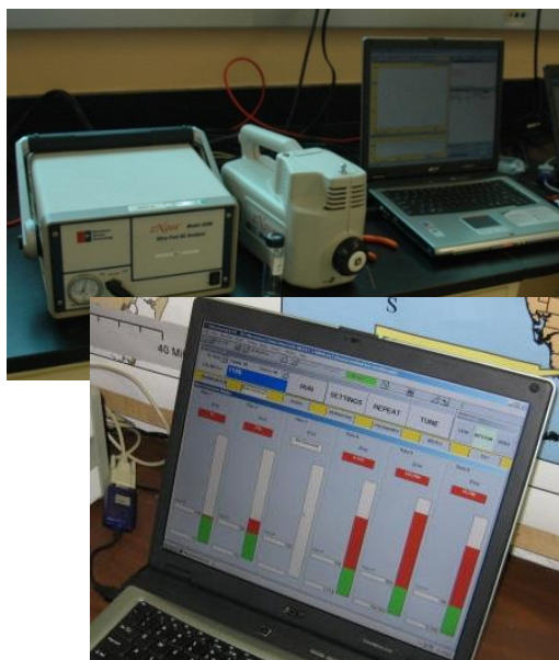
Computer graph indicating detection of five relevant specific VOCs
