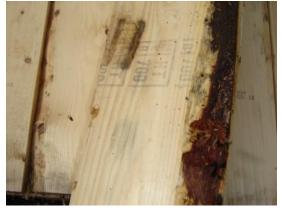
**Image 2** - Bark on edge of board is less than 3 cm wide therefore the board complies with bark tolerances.
