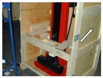
**Image 7** - Shipping crate Note the plywood identified by the arrow is exempt
