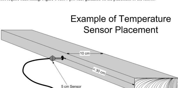
Some sensor designs (e.g. metal capped sensors) prevent the entry of air into the hole and therefore do not require back filling. Figure 6 below provides guidance on the placement of the sensor.
