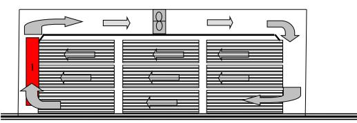
**Figure 3**: A heating chamber in which the heating pipes are located with a fan above the wood stack. The cold spot is likely to be nearest the exit side of the stack and the temperature sensor should be placed where the air exits the wood stack (marked "1").
