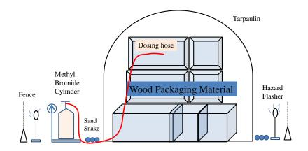
Figure 5. Common Layout of Tarpaulin Fumigation
