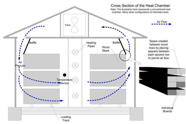
**Figure 2:** A type of heat chamber with the heating pipes in the middle. Temperature sensors should be placed at a location where the air exits the wood stack and is therefore likely to be the coolest.
