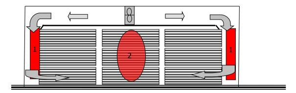
**Figure 4**: A heating chamber in which heating is bi-directional. If the treatment schedule is long, the cold spot may be at the air exit side of the wood (marked 1). Temperature sensors should be placed along the walls of the chamber. If the schedule is shorter, the cold spots are likely to be in center of the wood stack (marked "2") and sensors should be placed there.
