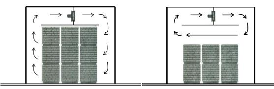
**Figure 1**: Schematic illustration of a loaded heat chamber resulting in different air circulation. Left: with a completely stockpiled chamber (cross section), the air circulates through the entire stack and heating is more uniform. Right: in an incompletely stockpiled chamber (cross section), the air circulates over the wood stack and the wood is not heated as quickly as the free space in the chamber.
