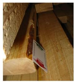
**Image 5** - Bark on the edge is wider than 3 cm and the piece is greater than 50 cm<sup>2</sup>. The bark must be removed or the piece may not be used in wood packaging material.
