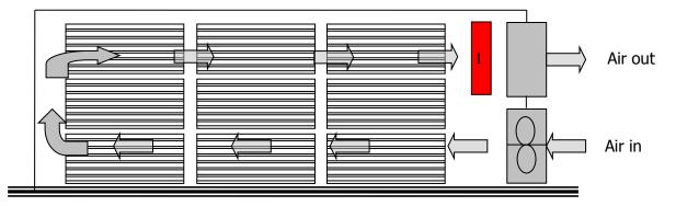
Figure 5: A heating chamber in which heating occurs at the floor of one-side. The temperature sensor is placed at the air exits the wood stack (marked "1").
