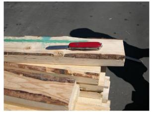
Image 3 - Bark on the edge of the board. The knife is 2 cm by 15 cm, therefore the board complies with tolerances. The board below the one with a knife, only contains wane (discoloured cambium) and is therefore compliant.
