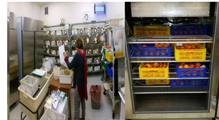
Peach fruit fly colonies and climatic chamber used for cold treatment evaluations.
