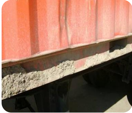
Soil contamination on external surface
