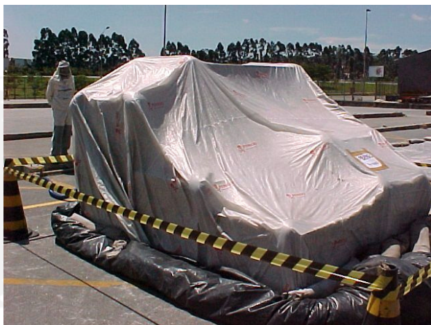
WOOD PALLETS AND BOXES RECEIVING METHYL BROMIDE UNDER PLASTIC COVER
