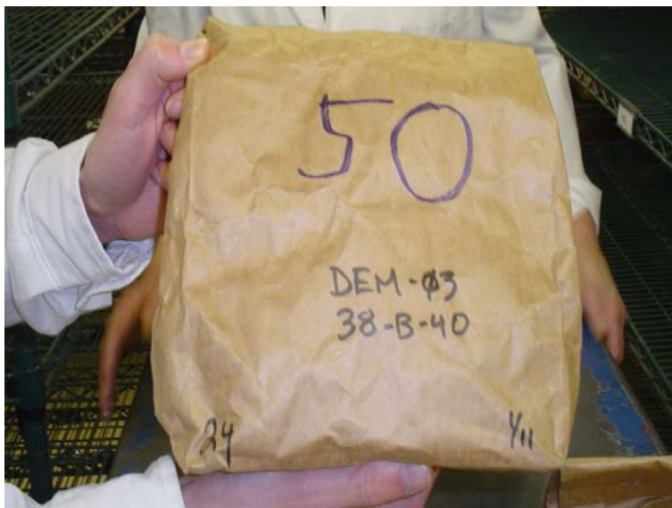
FIGURE 2-4-3 Sample Beaker Number (50), Collection Number (DEM-03), Field Name (38-B-40), Sample Bag Number (24), and Collection Date (1/11)
