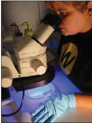
FIGURE 12.3 Ultraviolet light and dissection microscope combination for examining dyed fruit flies (Courtesy USDA and FDACS).
