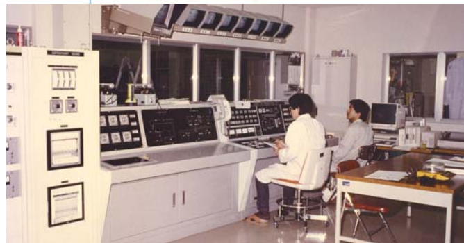
(5) Irradiation system control center (pupa-loading, transfer, irradiation, and unloading are monitored by computers to ensure safety and accuracy).
