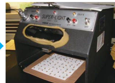
(b) The specimens on the filter paper are examined under ultra-violet light. The dye fluoresces when irradiated by ultra-violet rays.
