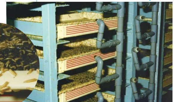
(5) Mature larvae leaving the trays (the larvae fall into the water and enter state of suspended animation)
