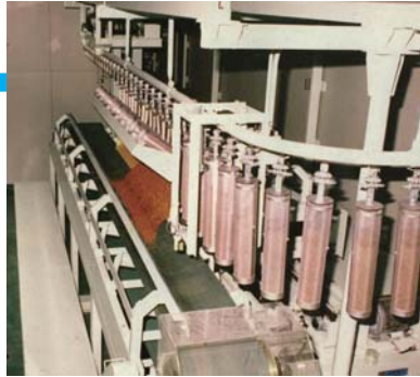
(3) Pupa-unloading equipment (irradiated pupae are unloaded and conveyed to the Sterile fly release center).
