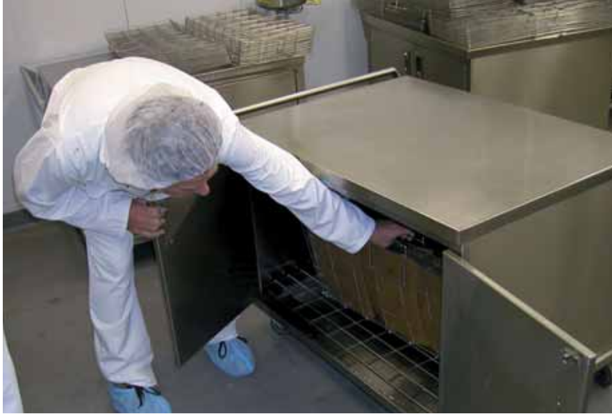
FIGURE 27 Stainless-steel cart, specially designed to hold disinfected egg sheets, for transporting egg sheets from the egg-sheet preparation room to the diet-dispensing room. (OKSIR facility, Osoyoos, Canada)
