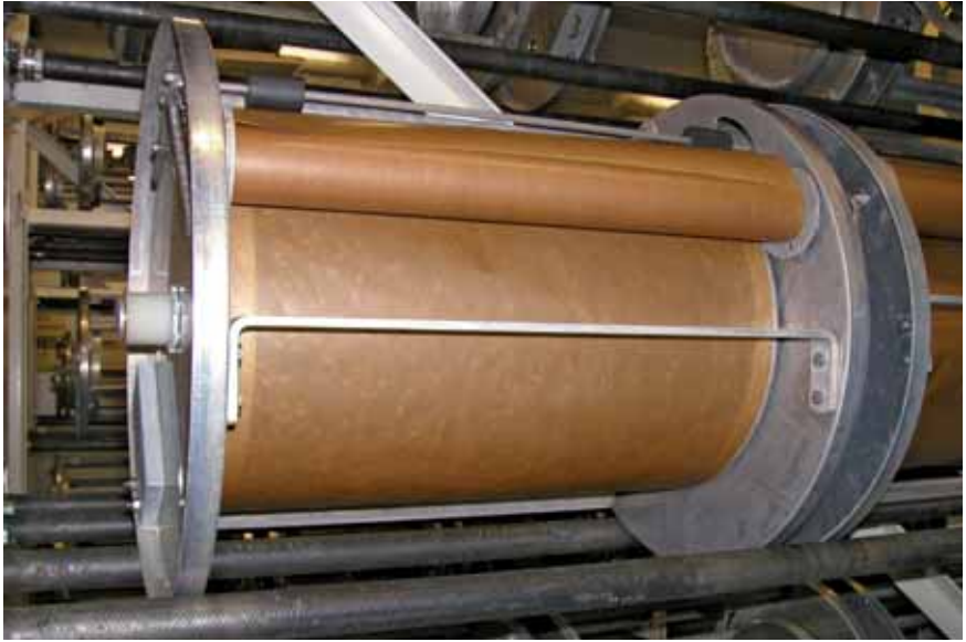
FIGURE 21 Oviposition cage resting on slowly turning rollers. Constructed from aluminium and using brown paper waxed on both sides (OKSIR facility, Osoyoos, Canada)
