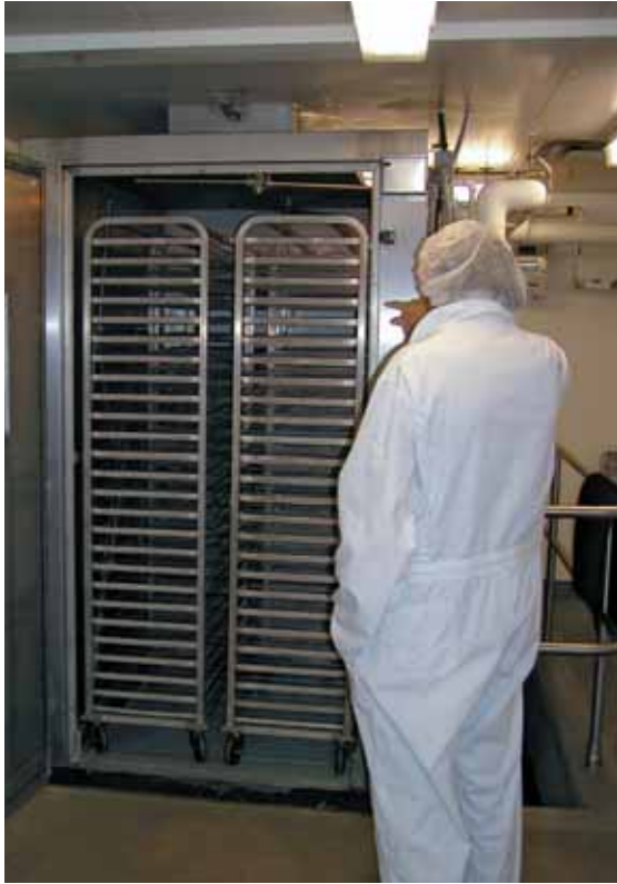
FIGURE 31 Cart washer (also used to wash oviposition cages) – OKSIR mass-rearing facility, Osoyoos, Canada
